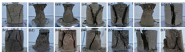
Fig.4. The development of shale samples behavior from ductile (for untreated compacted samples) to brittle (for stabilized samples): a) DB; a1) Natural compacted DB; a2) DB+CKD 7days; a3) DB+CKD 28days; a4) DB+CKD 90days; a5) DB+L/CKD 7days; a6) DB+L/CKD 28days; a7) DB+L/CKD 90days; b) DQ; b1) Natural compacted DQ; b2) DQ+CKD 7days; b3) DQ+CKD 28days; b4) DQ+CKD 90days; b5) DQ+L/CKD 7days; b6) DQ+L/CKD 28days; b7) DQ+L/CKD 90days.
